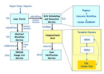
Fig. 2. The distributed architecture of the Montage TeraGrid Portal.
