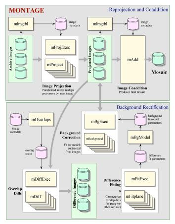
Fig. 1. The high-level design of Montage.
