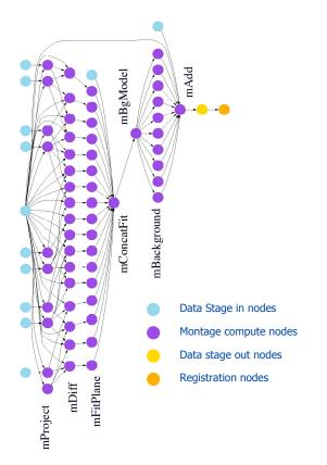
Fig. 5. Example concrete (executable) workflow for a 10 input file job on a single cluster. In addition to the computation nodes, the concrete workflow includes nodes for staging data into and out of the computation and for registering the data products for later retrieval.
