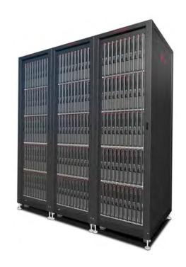
A Linux Networx Custom Supersystem will be the next-generation supercomputer for the NASA Center for Computational Sciences. The first stage of the cluster, providing 3.3 teraflops of peak computing power in five closet-sized cabinets, will arrive in June (Photo credit: Linux Networx).
