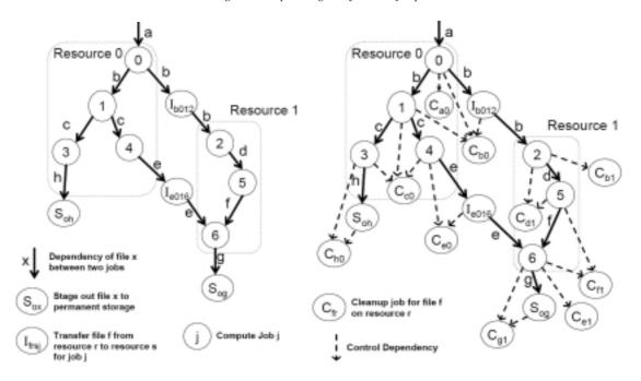
Fig. 2. (a) The original executable workflow mapped by Pegasus to two resources. (b) The workflow with dynamic cleanup nodes added.
