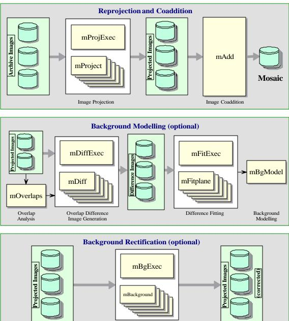
Figure 2: Design Components of Montage - Process Flow Overview.
